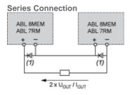
(1) Two Shottky diodes Imin = power supply In and Vmin = 50 V
