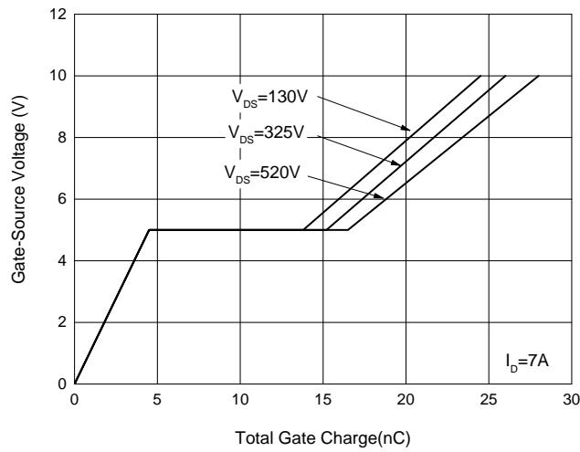
Fig. 6 - Gate-Source Voltage Characteristics
