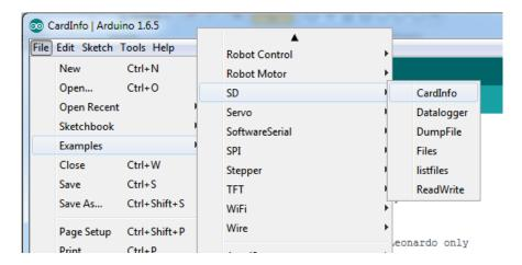
Luckily many of the default examples already have **chipSelect** = **4** For other sketches, do check to make sure that CS is set to 4! The SD card uses hardware SPI for the remaining pins.
