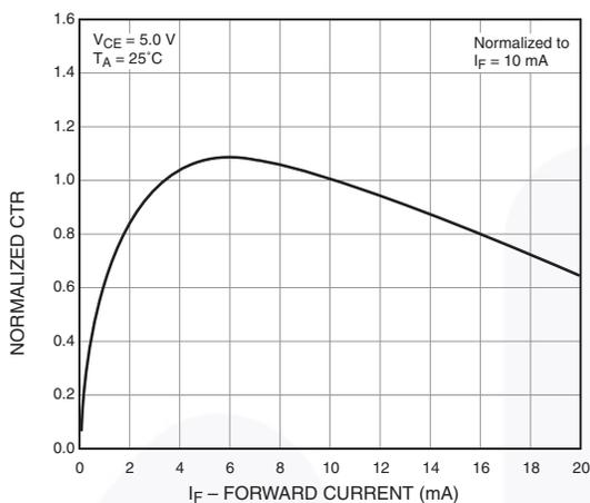
Figure 3. Normalized CTR vs. Forward Current
