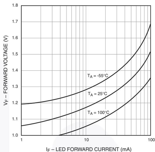
Figure 10. LED Forward Voltage vs. Forward Current
