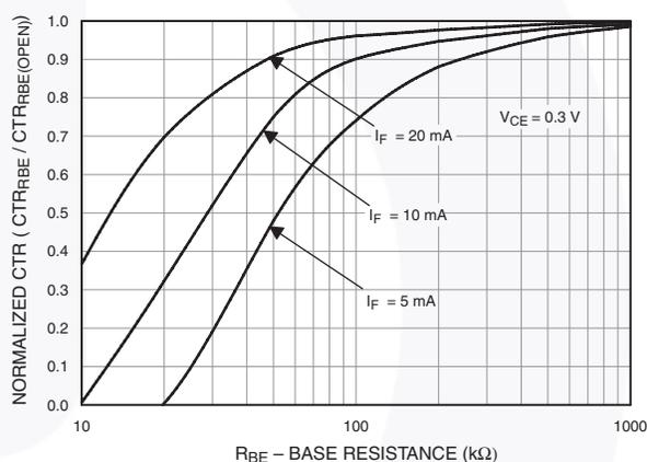
Figure 6. CTR vs. R<sub>BE</sub> (Saturated)
