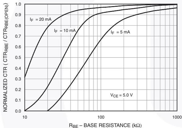
Figure 5. CTR vs. R<sub>BE</sub> (Unsaturated)
