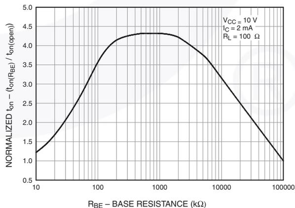
Figure 8. Normalized  $t_{on}$  vs. R<sub>BE</sub>
