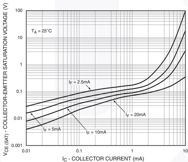
Figure 11. Collector-Emitter Saturation Voltage vs. Collector Current
