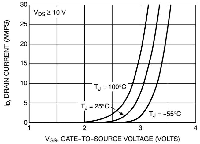
Figure 2. Transfer Characteristics
