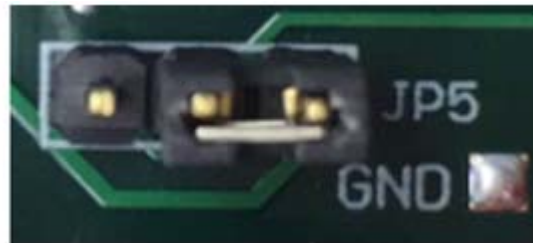
Figure 2B. (JP5: Pin 2 - 3 to Banana Jack)
