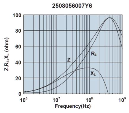
Impedance, reactance, and resistance vs. frequency.
