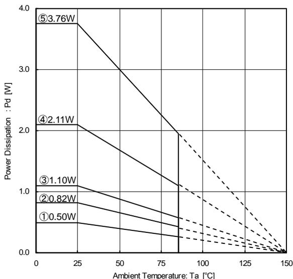
Measure condition: mounted on a ROHM board, and IC
