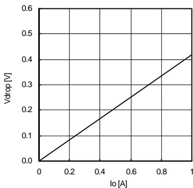
Fig.34 Minimum dropout Voltage3
