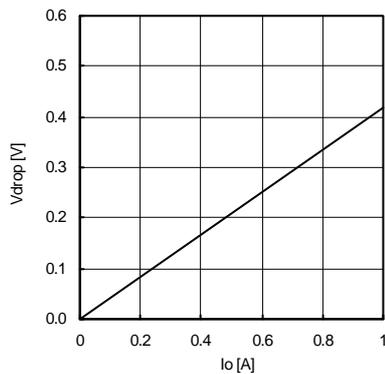
Fig.35 Minimum dropout Voltage4
