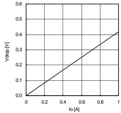
Fig.33 Minimum dropout Voltage2
