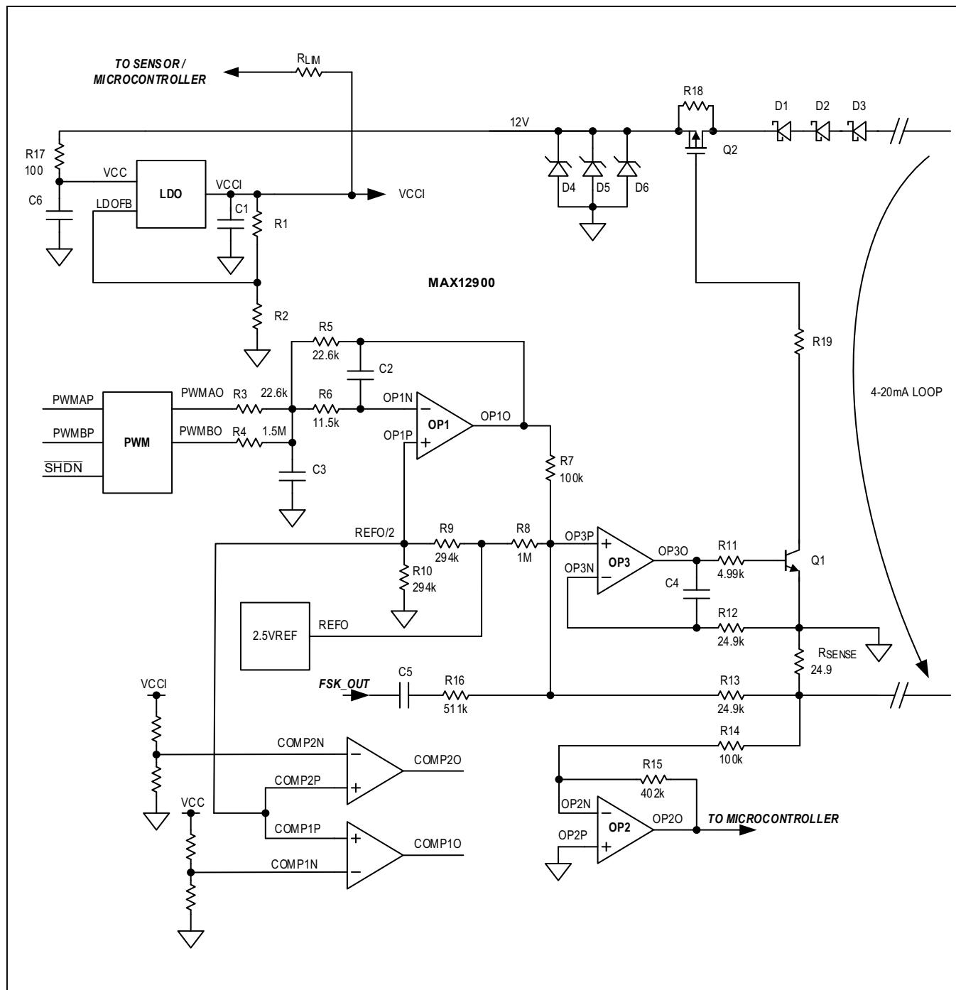
Figure 4. Loop-Powered 4-20mA Transmitter for Hazardous Environments
