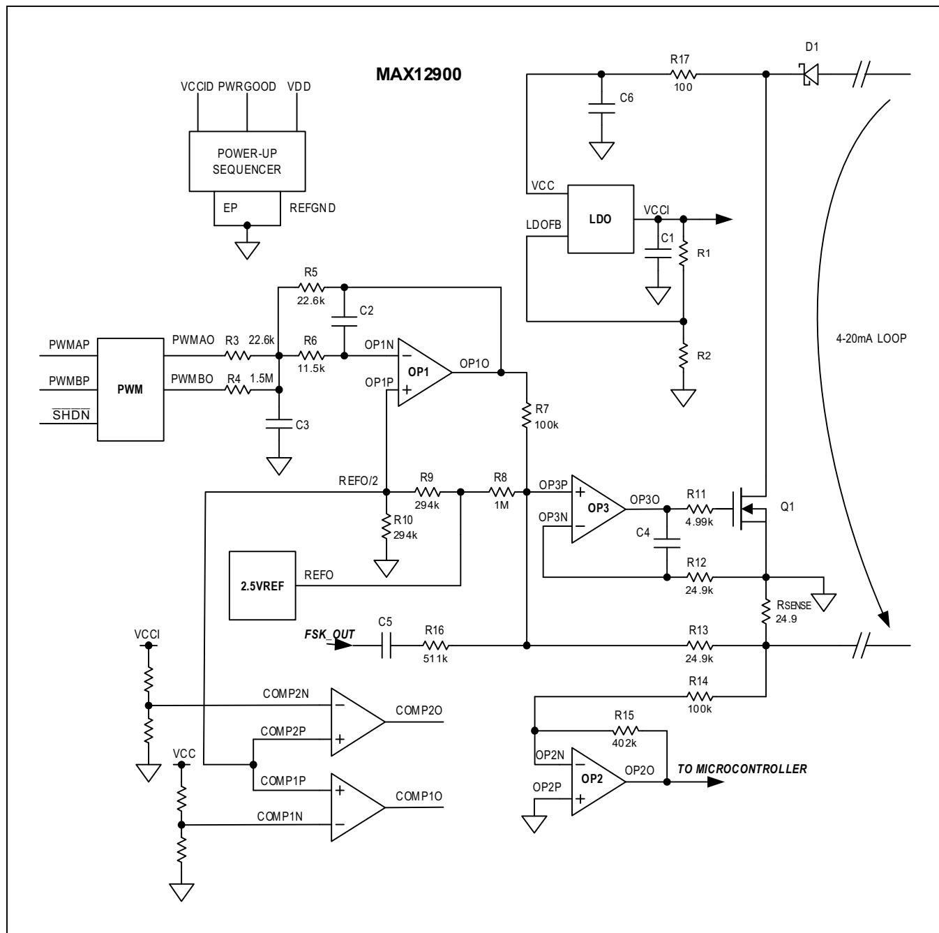
Figure 2. Loop-Powered 4-20mA Transmitter with Two PWM Inputs
