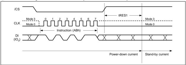
Figure 38a. Release Power-down Instruction (SPI Mode)
