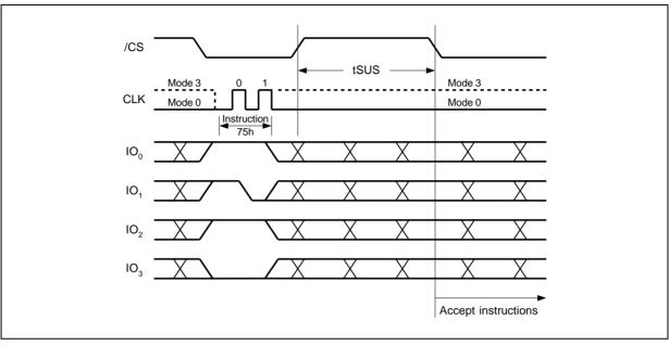
Figure 35b. Erase/Program Suspend Instruction (QPI Mode)
