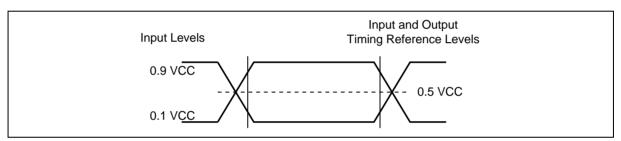
Figure 59. AC Measurement I/O Waveform
