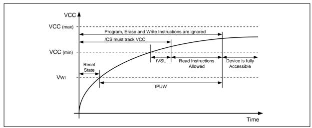
Figure 58a. Power-up Timing and Voltage Levels
