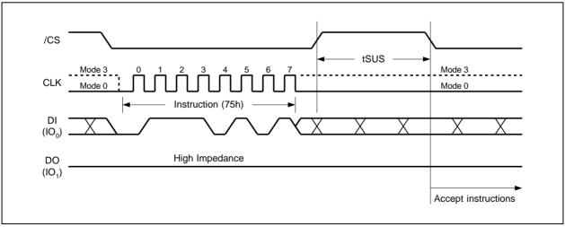
Figure 35a. Erase/Program Suspend Instruction (SPI Mode)
