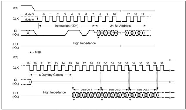
Figure 17a. DTR Fast Read Instruction (SPI Mode)
