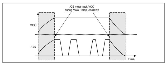
Figure 58b. Power-up, Power-Down Requirement
