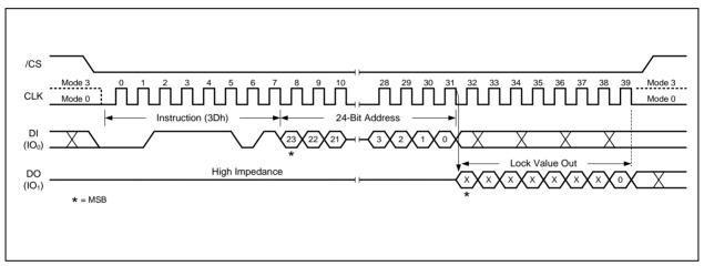
Figure 55a. Read Block Lock Instruction (SPI Mode)
