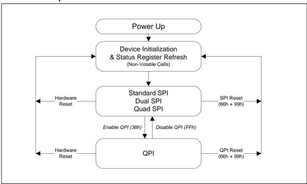
Figure 3. W25Q128JV Serial Flash Memory Operation Diagram
