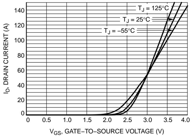
Figure 2. Transfer Characteristics
