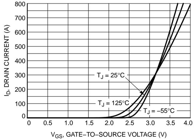
Figure 2. Transfer Characteristics
