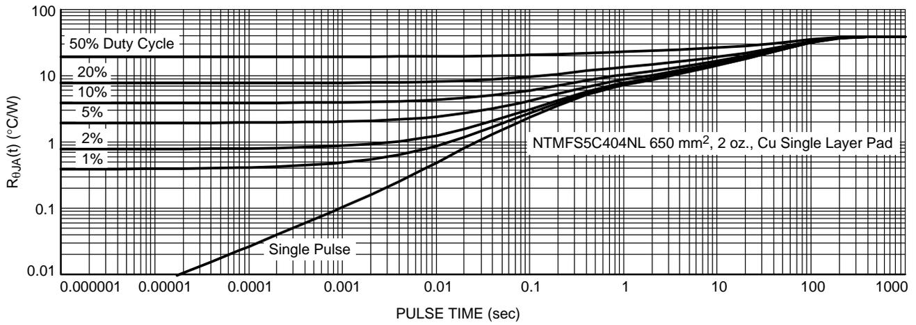
Figure 13. Thermal Characteristics
