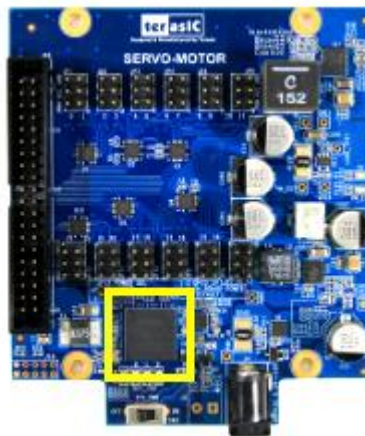
Figure 2-12 CPLD for Power Monitor
