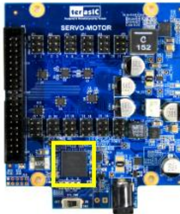
Figure 2-12 CPLD for Power Monitor
