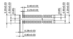
Recommended metal mask opening pattern Metal mask thickness: When 120µm (Terminal opening ratio: 70%) (Metal-part opening ratio: 100%)
