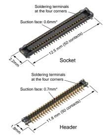
\* Suction face size for the 1.0 mm/1.5 mm mated height type: Socket — 0.64 mm, Header — 0.76 mm
