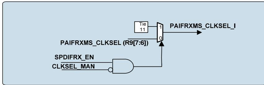
Figure 36 Manual Clock Over-ride of PAIF Rx
