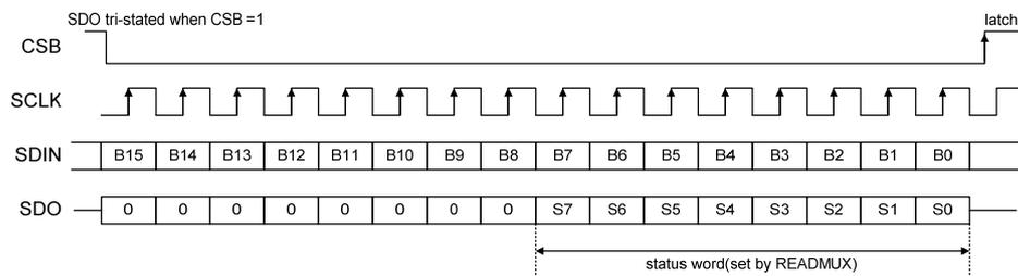
Figure 7 3-Wire SPI Compatible Interface Continuous Readback
