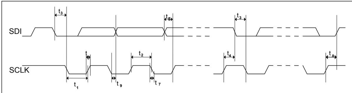
**Figure 5 Control Interface Timing – 2-Wire Serial Control Mode**
