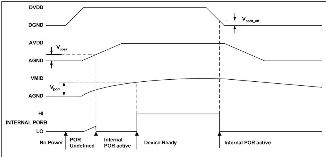
Figure 41 Typical Power up Sequence where DVDD is Powered before AVDD
