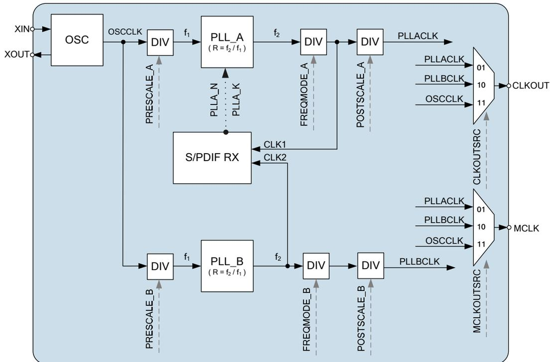
Figure 38 PLL and Clock Select Circuit
