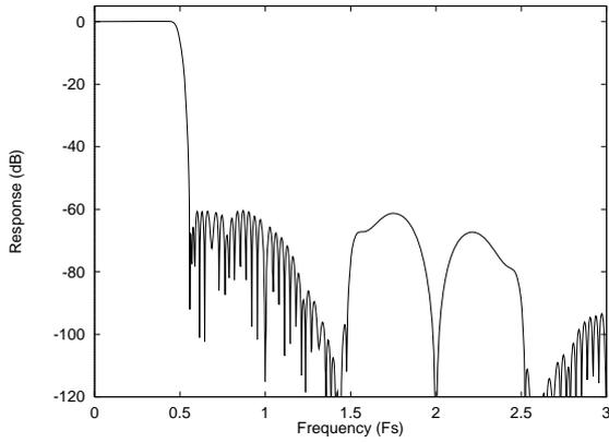
Figure 43 DAC Digital Filter Frequency Response – 44.1, 48 and 96kHz
