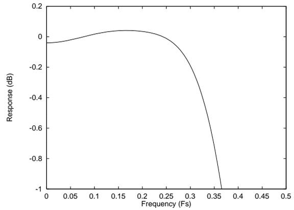
Figure 46 DAC Digital Filter Ripple – 192kHz
