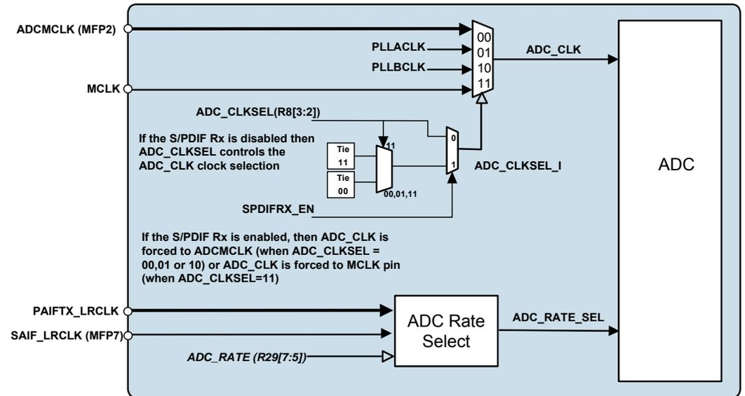
**Figure 27 ADC Clock and ADC Rate Selection**
