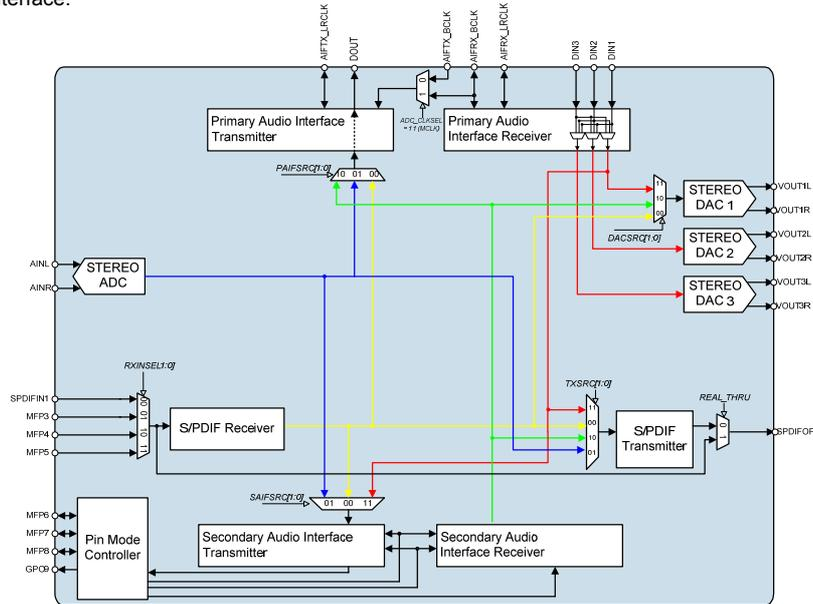
Figure 25 Digital Routing
