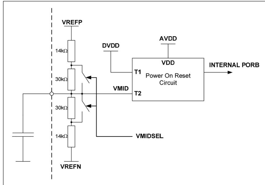
**Figure 40 Internal Power On Reset Circuit Schematic**
