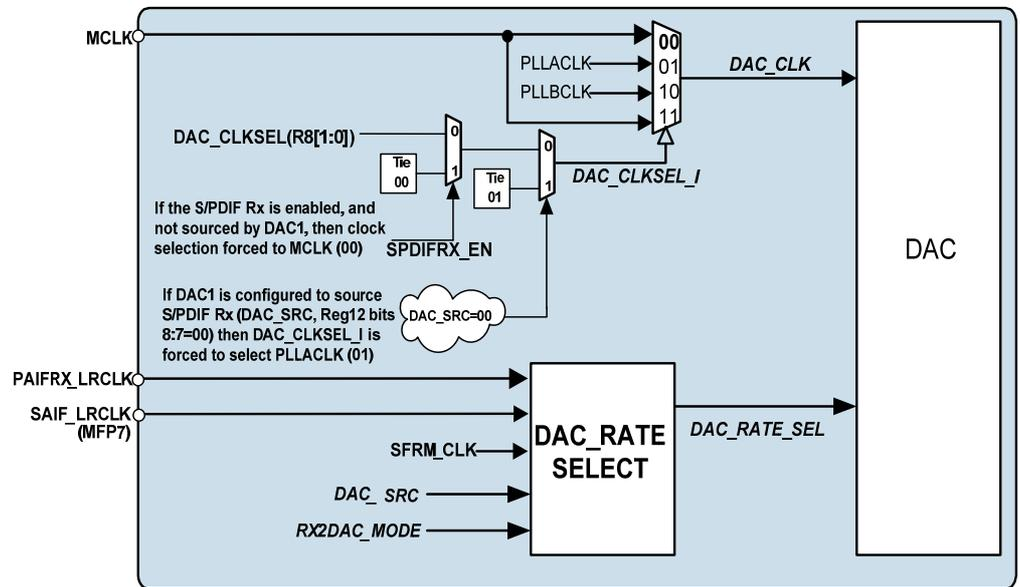
Figure 26 DAC Clock and DAC Rate Selection
