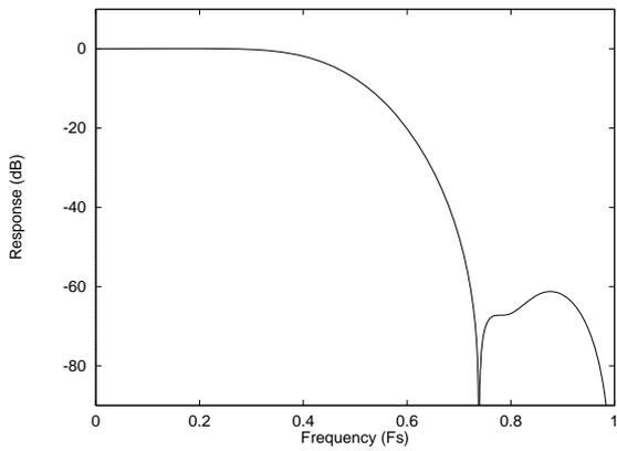
Figure 45 DAC Digital Filter Frequency Response – 192kHz
