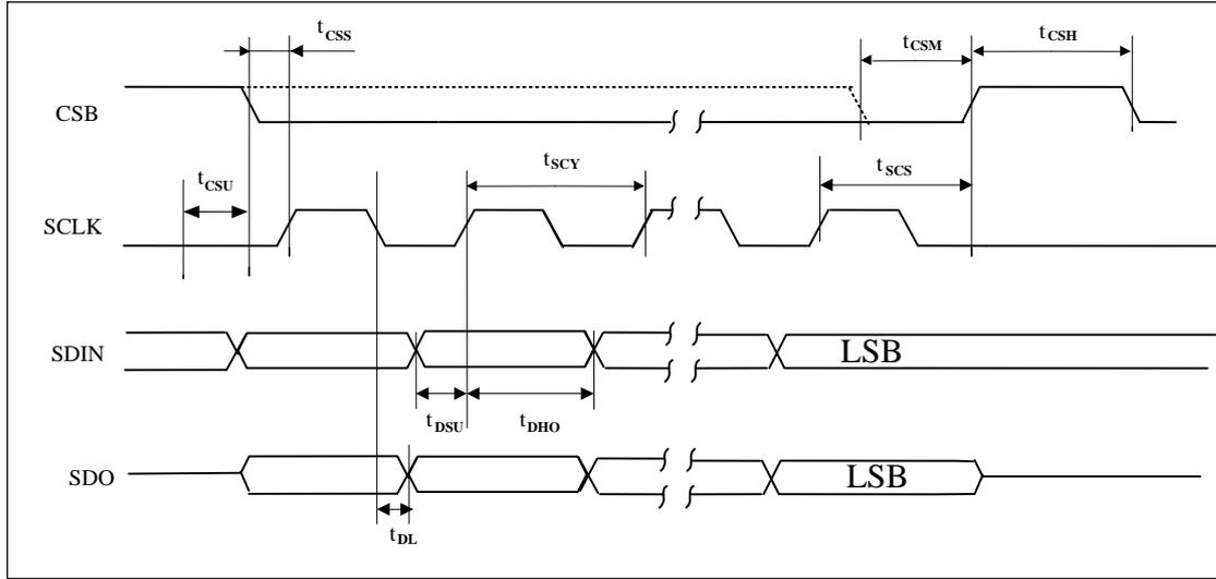
**Figure 4 SPI Compatible Control Interface Input Timing**
