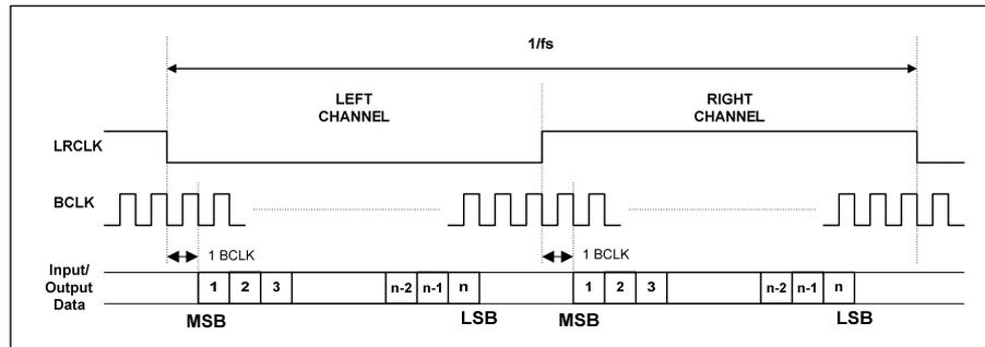
Figure 16 I<sup>2</sup>S Mode Timing Diagram
