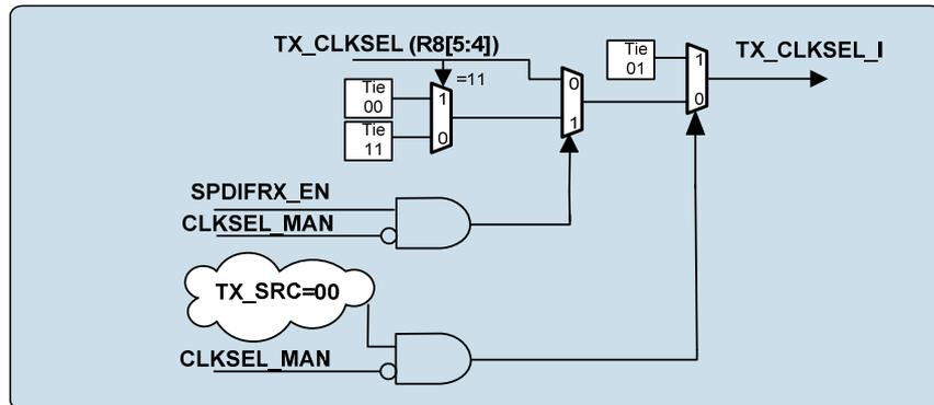
Figure 34 Manual Clock Over-ride of S/PDIF Tx Clock
