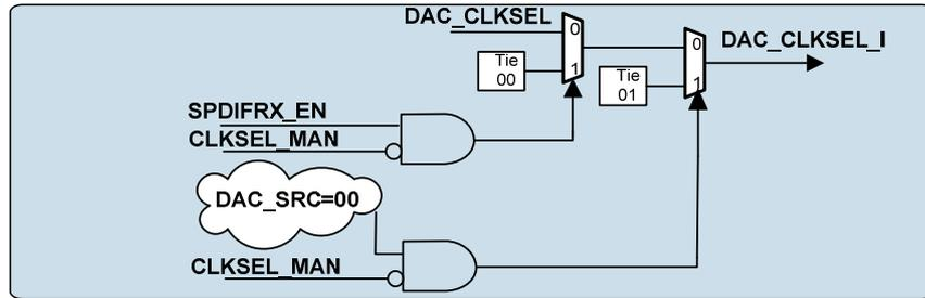
Figure 32 Manual Clock Over-ride of DAC Clock
