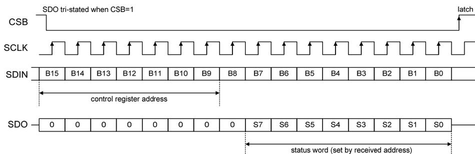
**Figure 8 3-Wire SPI Compatible Control Interface Non-Continuous Readback**
