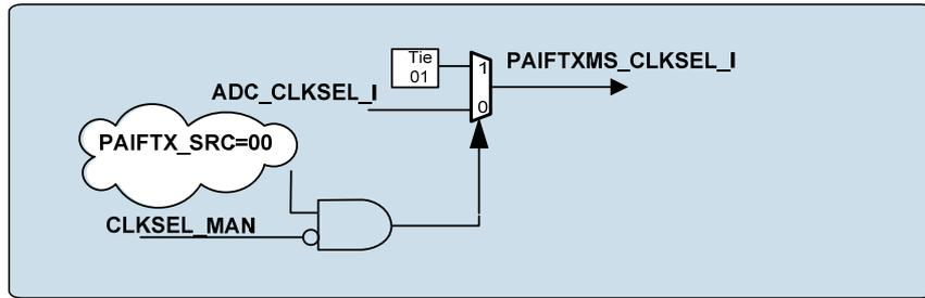
Figure 35 Manual Clock Over-ride of PAIF Tx
