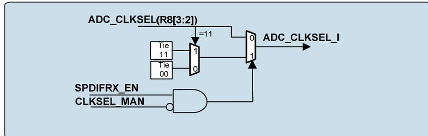
Figure 33 Manual Clock Over-ride of ADC Clock
