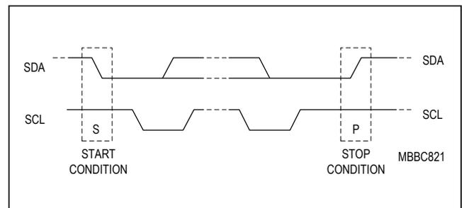
Figure 19. I<sup>2</sup>C Start and Stop
