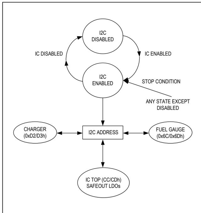
Figure 17. I<sup>2</sup>C Slave Address Structure
