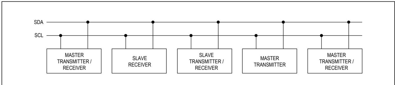
Figure 20. I<sup>2</sup>C System Configuration
