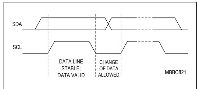
Figure 18. I<sup>2</sup>C Bit Transfer
