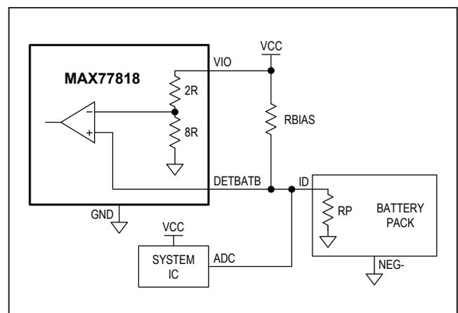
Figure 3. DETBATB Internal Circuitry and System Diagram
