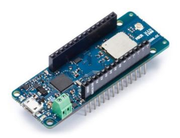
**Arduino MKR WAN 1300** has been designed to offer a practical and cost effective solution for makers seeking to add Lo-Ra connectivity to their projects with minimal previous experience in networking. It is based on the Atmel SAMD21 and a Murata CMWX1ZZABZ Lo-Ra module.
