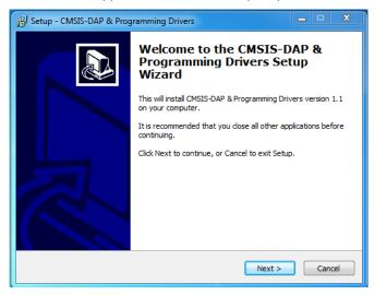
2. During the installation, a warning may appear that the publisher cannot be verified, depending on Windows security settings. Select, 'install this driver software anyway.' Two drivers are being installed, cmsis-dap and usbdirect.
