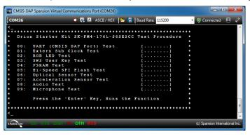
5. To run each of the tests enter the number next to the test description and follow the prompts. For example: 6<enter> will run the Optical Sensor Test. The application will output the value of the sensor and loop until the enter key on the PC keyboard is pressed.
