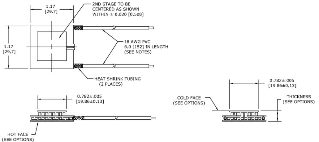
Ceramic Material: Alumina ( $\text{Al}_2\text{O}_3$ )
