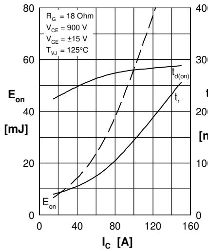
Fig. 4 Typ. turn-on energy & switch. times vs. collector current
