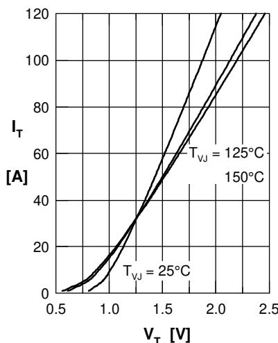
Fig. 1 Forward characteristics
