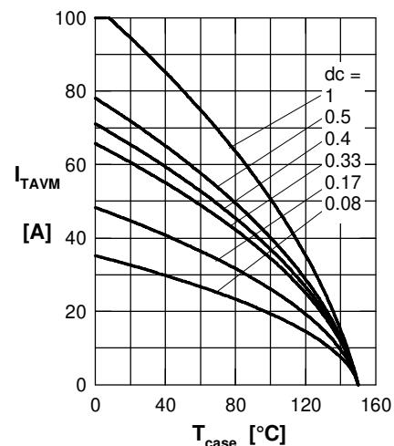
Fig. 6 Max. forward current at case temperature
