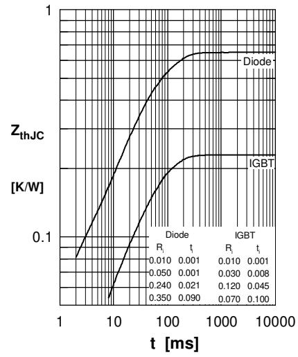
Fig. 9 Transient thermal resistance junction to case
