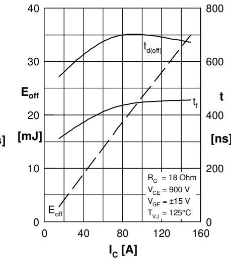
Fig. 5 Typ. turn-off energy & switch. times vs. collector current
