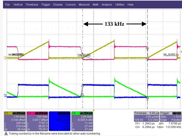
Figure 62. Rated Load [2 us/div]
