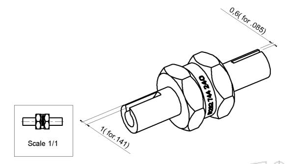
USE THIS TOOL TO POSITION THE CABLE CORRECTLY INTO THE CONNECTOR FOR SOLDERING.
