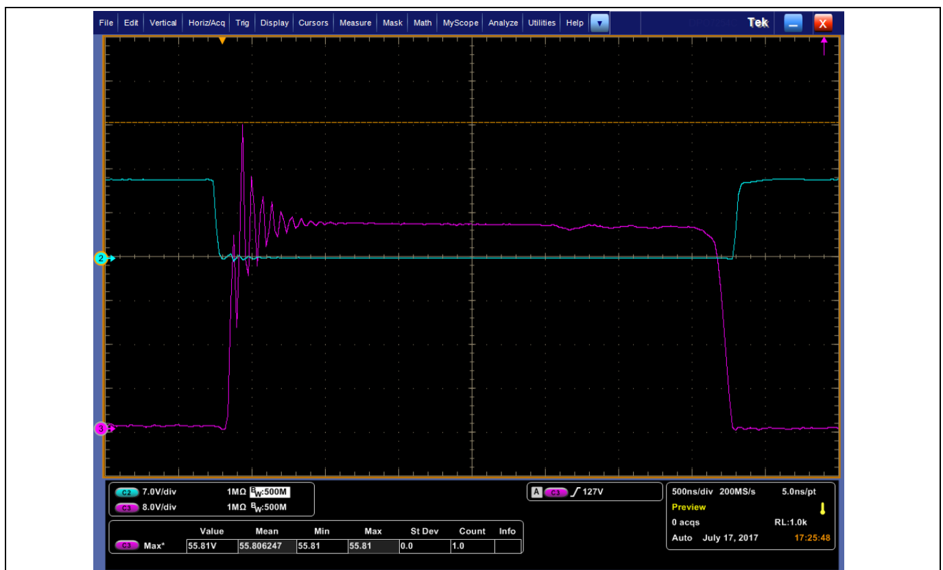
Figure 64 Synchronous turn-on/off delay at 140 W load. V_{DS} (purple) and V_{GS} (blue).
