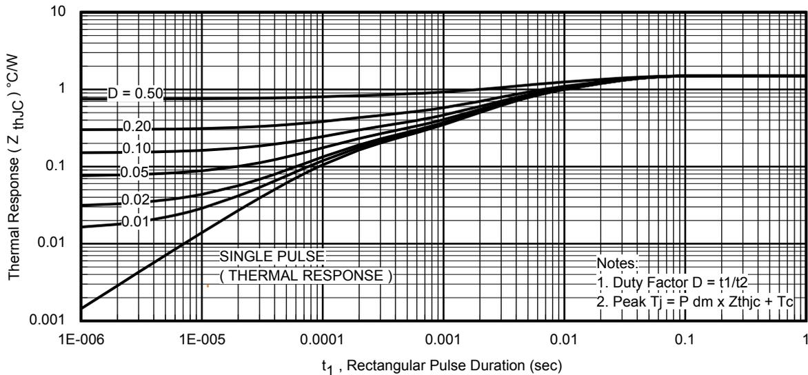
**Fig 14. Maximum Effective Transient Thermal Impedance, Junction-to-Case**
