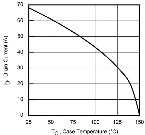
**Fig 2.** Maximum Drain Current vs. Case Temperature
