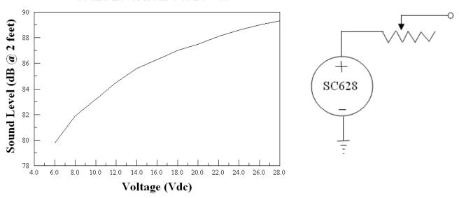
It was verified that the circuitry of model SC628R is not affected by a potentiometer, so data was gathered to find the value of a potentiometer that gives the greatest range of sound change.
