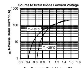
V<sub>SD</sub>, Source to Drain Voltage (V)
