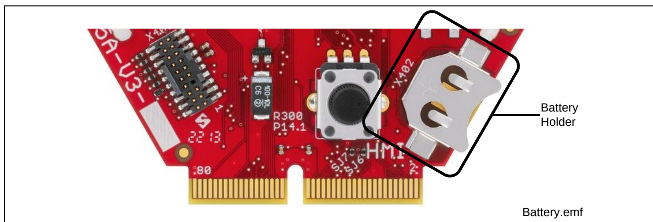
Figure 5 Battery (VBAT Supply)
