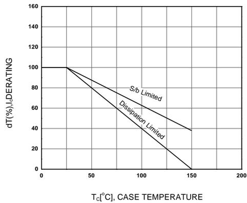
Figure 6. Derating Curve of Safe Operating Areas
