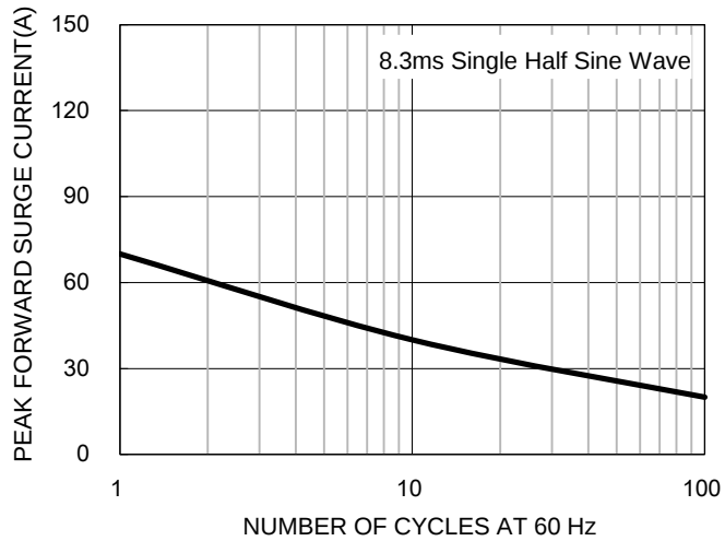
Fig.5 Maximum Non-repetitive Forward Surge Current
