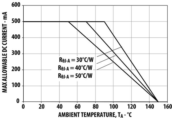
**Figure 22 Maximum Pulse Current vs. Ambient Temperature.**
