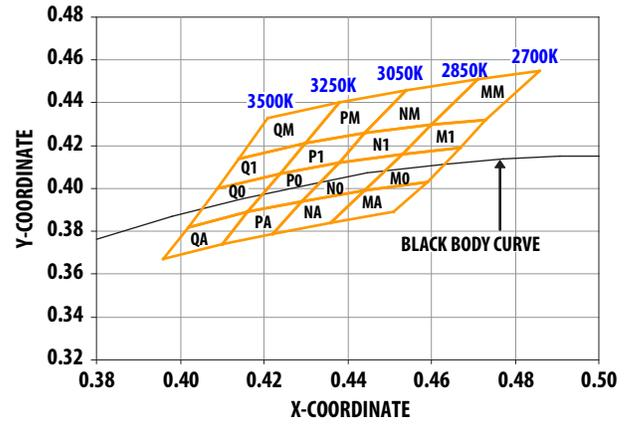
Figure 4 Color Bin Structure for Neutral White
