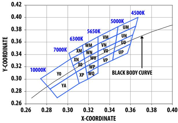
Figure 3 Color Bin Structure for Warm White
