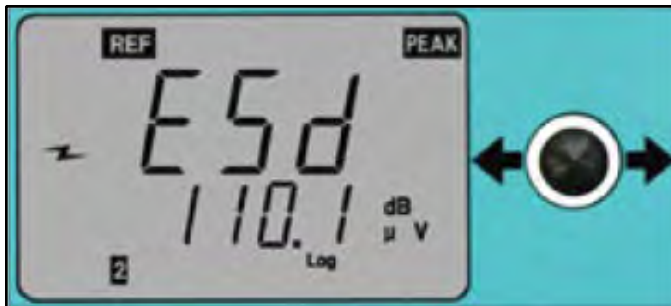
Figure 7. Modifying the ESD event threshold
