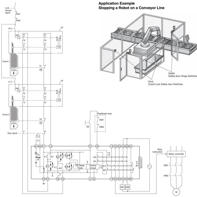
S1: Safety-door Switch with direct opening contact
