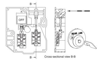
(4) Operation Key inserted, solenoid ON, and trapped key inserted. Status: Door locked and trapped key can be removed.
