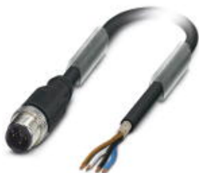
Sensor/actuator cable, 4-position, PUR halogen-free, black-gray RAL 7021, shielded, Plug straight M12, A-coded, on free cable end, cable length: 1 m
