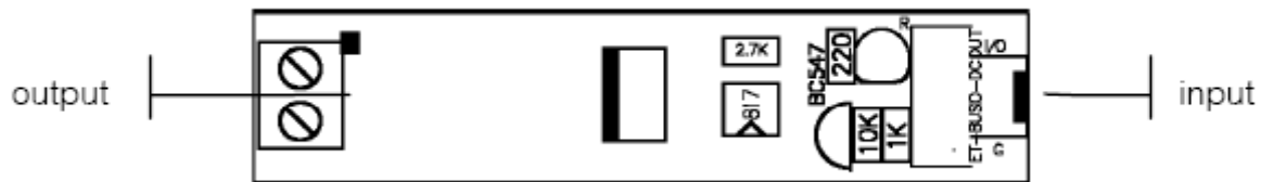
FIG 1: MR-BusIO-DCOUT Board Layout
