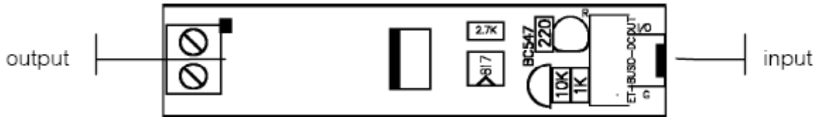
FIG 1: MR-BusIO-DCOUT Board Layout
