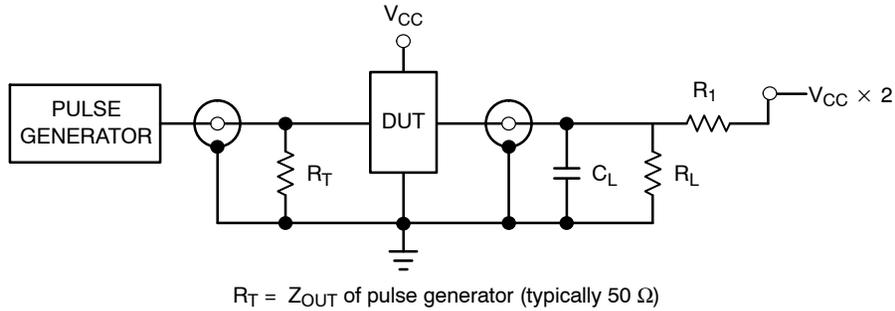
Figure 4. Test Circuit
