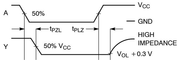
Figure 3. Switching Waveforms
