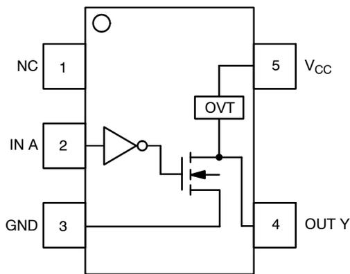
Figure 1. Pinout
