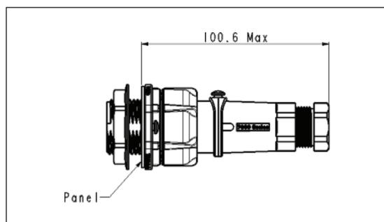
Mated dimensions - Flex connector to in-line connector
