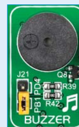
Figure 18-2: Use jumper J21 to connect Piezo buzzer on PB1 or PD4 pin
