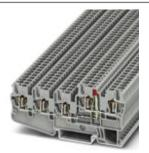
Sensor/actuator terminal block, Connection method: Spring-cage connection, Cross section: 0.08 mm² - 4 mm², AWG: 28 - 12, Width: 5.2 mm, Color: gray, Mounting type: NS 35/7,5, NS 35/15
