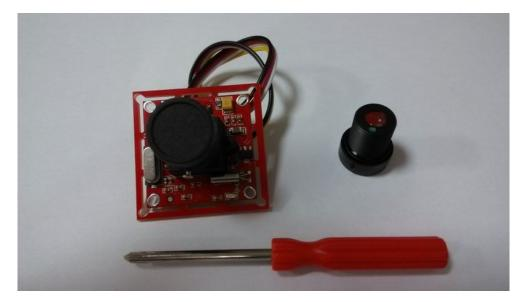
Then, unscrew the screws on the side of lens:
