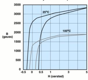
Measured on a 17/10/6mm toroid at 10kHz.
