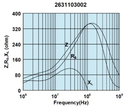
Impedance, reactance, and resistance vs. frequency.
