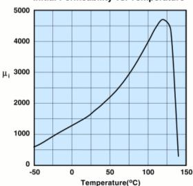
Measured on a 17/10/6mm toroid at 100kHz.
