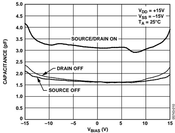
Figure 21. Capacitance vs. Source Voltage for Dual Supply
