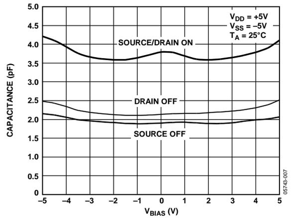
Figure 23. Capacitance vs. Source Voltage for Dual Supply
