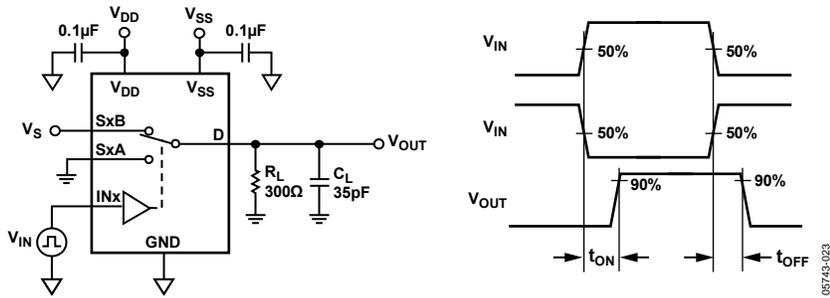
Figure 27. Switching Timing
