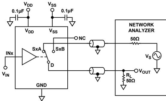
$$\text{INSERTION LOSS} = 20 \log \frac{V_{OUT \text{ WITH SWITCH}}}{V_{OUT \text{ WITHOUT SWITCH}}}$$
