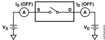
Figure 25. Off Leakage
