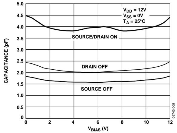
Figure 22. Capacitance vs. Source Voltage for Single Supply
