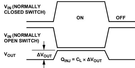
Figure 30. Charge Injection
