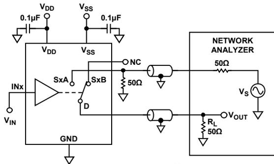
$$\text{OFF ISOLATION} = 20 \log \frac{V_{OUT}}{V_S}$$
