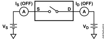
Figure 25. Off Leakage
