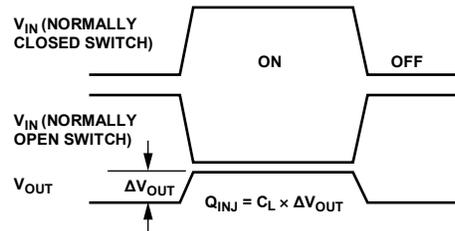
Figure 30. Charge Injection
