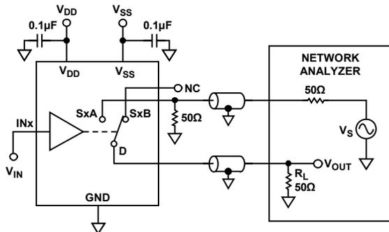
$$\text{OFF ISOLATION} = 20 \log \frac{V_{OUT}}{V_s}$$
