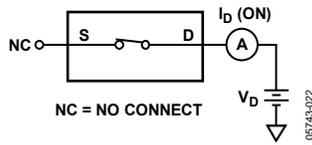
Figure 26. On Leakage
