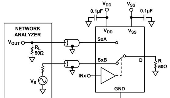
$$\text{CHANNEL-TO-CHANNEL CROSSTALK} = 20 \log \frac{V_{OUT}}{V_s}$$
