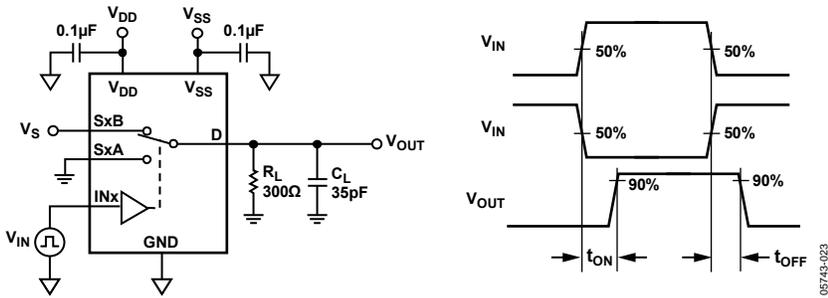
Figure 27. Switching Timing
