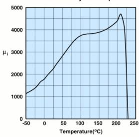
Measured on an 18/10/6mm toroid at 100kHz.
