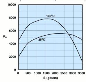
Measured on an 18/10/6mm toroid at 10kHz.
