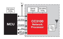
The CC3100 device is a Wi-Fi, self-contained network processor with on-chip web server and embedded TCP/IP stack that connects easily to any low-cost and low-power microcontroller (MCU) such as the MSP430F552, thanks to a simple UART or SPI driver and host memory footprint as low as 7kB of code to reside on the MCU. Hardware design is made easy for space-constrained boards with a small 64-pin 9×9 mm QFN package. Certified modules will
