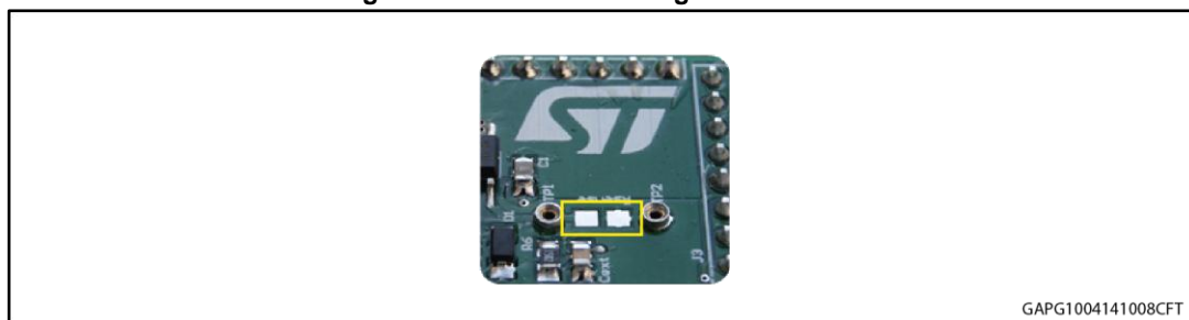
Figure 5: Pads for soldering SMD resistor
