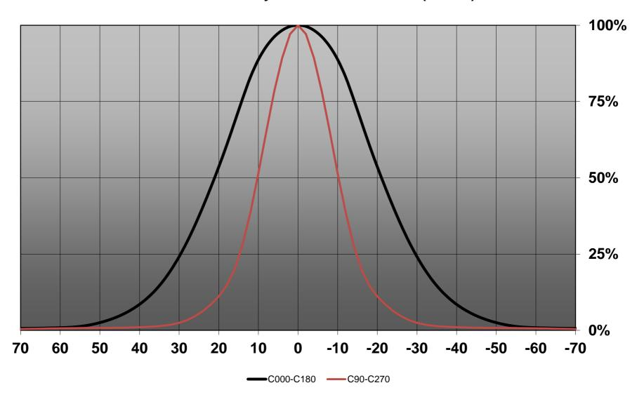
Luminaire: Ledil Oy FA11912\_CXM\_O FA11912\_CXM\_O Lamps: 1 x Cree XM-L white
