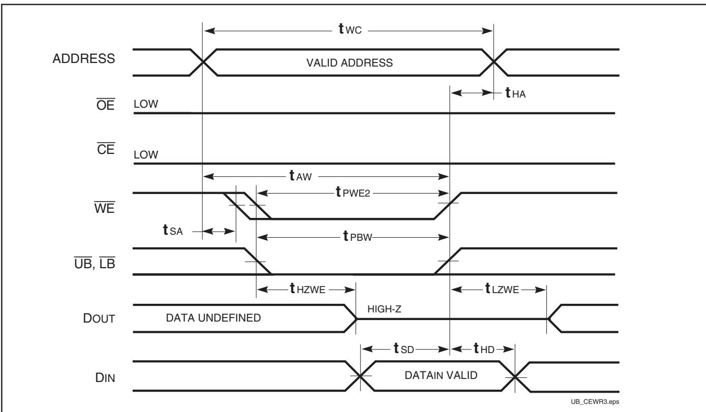
WRITE CYCLE NO. 4 ( $\overline{LB}$ ,  $\overline{UB}$  Controlled, Back-to-Back Write)<sup>(1,3)</sup>
