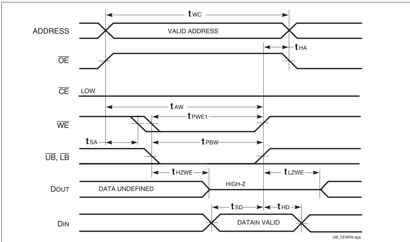
WRITE CYCLE NO. 3 ( $\overline{WE}$  Controlled:  $\overline{OE}$  is LOW During Write Cycle)
