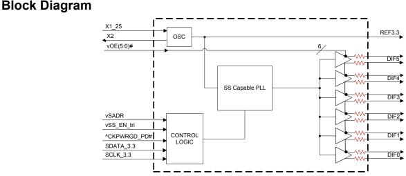
Note: Resistors default to internal on 41/51 devices. P1 devices have programmable default impedances on an output-by-output basis.
