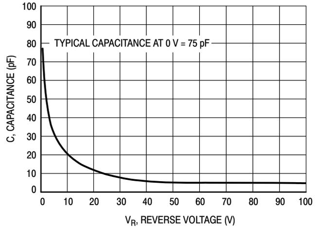
Figure 10. Typical Capacitance
