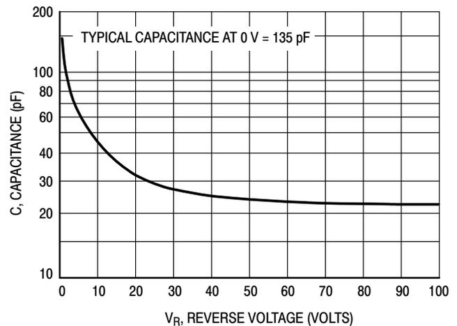
Figure 5. Typical Capacitance
