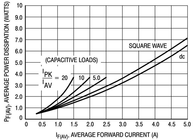
Figure 8. Power Dissipation
